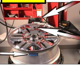
**5** Position valve hole at 12 o'clock (under tire machine mounting head) and mount the bottom tire bead.
