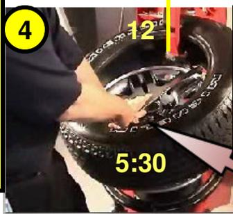
**4** Reposition valve hole at 5:30 and dismount bottom tire bead.
