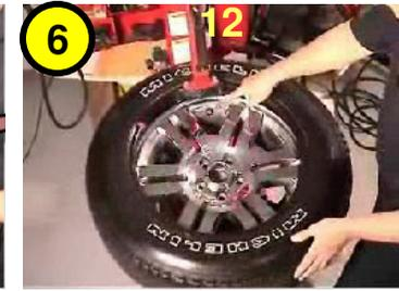
**6** Reposition valve hole at 12 o'clock and mount top tire bead.
