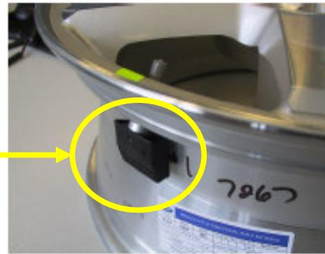
Remove retaining nut. Do not remove the valve stem core to relieve the tire pressure.
