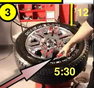
**3** Position valve hole at 5:30 position relative to machine arm at 12 o'clock and dismount top tire bead.
