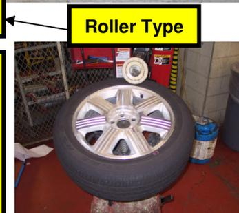
Do not allow the tire beads to move beyond the wheel mid-plane (middle of the wheel) when separating the beads from the wheels or damage to the TPMS sensor may occur.
